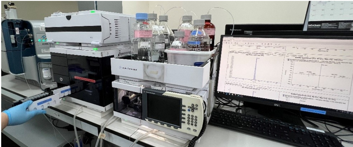
Photo 10: Loading of sample extracts into LC-MS for confirmatory test
